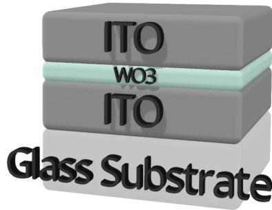
Figure 10: Final Design Device level schematic
